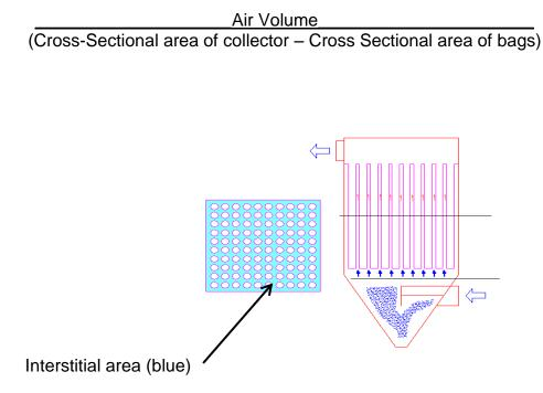
The optimal interstitial velocity is a function of several variables. They include bulk density, particle size distribution, agglomerating/non-agglomerating tendencies of the dust and inlet loadings.
