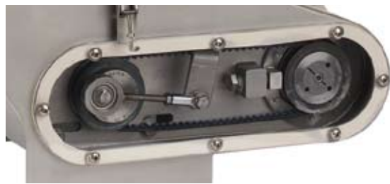
Quiet running clogged belt drive and robust drive construction.
