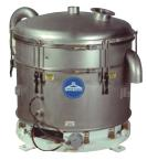
PSI<sup>™</sup>. The pneumatic Sweco In-line Sifter is used to sift dry flowing material. It can also be used to segregate smaller particles from larger particles, and to remove foreign matter. It screens dry material only while being pneumatically conveyed. The PSI sifter includes an air by-pass system to provide equal pressure on both sides of the screening surface. Typical applications include: flour, starch, salt, sugar, and plastics.
