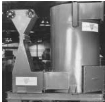
Often a hot gas stream has a valuable particulate to be recovered. Silver is recovered from film incineration using this Venturi scrubber.
