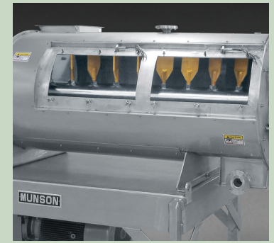
Model VIM-306-SS Variable-Intensity Continuous Blender constructed of stainless steel is equipped with a high-pressure vessel jacket to ASME code for heating or cooling. Shown with 180° adjustable paddles for varying degrees of blending intensity. Welded paddles (left) for sanitary service also available. Shown with doors removed.
