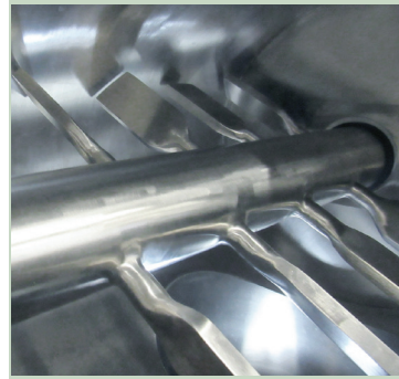
Large-radius ground and polished welds connecting paddles to the solid shaft eliminate crevices where materials could lodge, allowing rapid cleaning and sanitizing. For non-sanitary applications, the shaft can be equipped with 180° adjustable paddles (right) for varying degrees of blending intensity.
