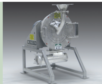
This 18 inch (457 mm) diameter Pin Mill model CIM-18-SS provides coarse to fine (400 mesh) grinding of friable materials into controlled particle sizes, as well as de-agglomerating and conditioning of dry solids. A direct drive system reduces the unit's footprint to about half of that required by a belt driven machine.
