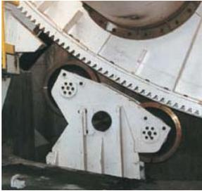
b) Reduces fatigue loading of each cycle on the end ring, thus increasing dumper life four fold.
