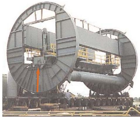
**Benefit:** The integral weigh platen allows cars to be weighed before and after dumping without the need of separate
