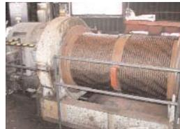
**Benefit:** Significantly improves wear life and durability by replacing the hoist drum with a new hard groove drum (or modifying existing drum to accept hard groove lagging) and cable is upgraded to IWRC
