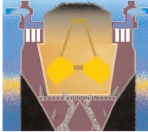
**Benefit:** Minimizes dust generation at its source and requires less ductwork, CFM and HP. Thus, costs less to install, operate and maintain than conventional bag house type systems.
