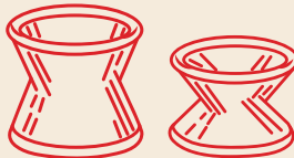
With the upper end fixed, the lower end is rotated, gradually reducing the orifice.
