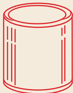
Diaphragm (nylon or other material) with retaining ring at each end.
