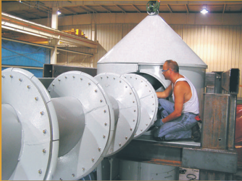
Each reclaim system is pre-assembled and power-tested prior to installation.
