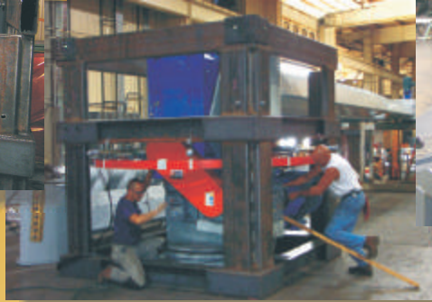
Each reclaim system is pre-assembled and power-tested prior to installation.
