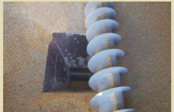
Near-total clean out is achieved with the reversible reclaim sweep auger, allowing the final clean-out cycle to be made in reverse.
