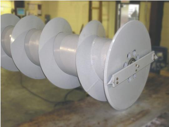
Laidig's innovative cupped flighting provides sharp, curved edges to maximize cutting and conveying efficiency, while also reducing starting torque and minimizing advance resistance.
