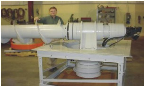
The low-profile dual-speed hydraulic reclaim drive system is compact and powerful, delivering high-torque with minimum material contact with the drive system.
