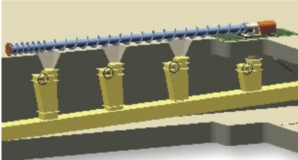
High-volume discharge is achieved by combining free-flow through draw downs with consistent high-delivery from the reclaim auger.
