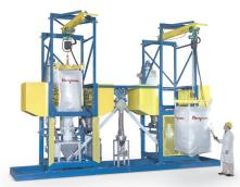
Bulk Bag Discharging Systems can loosen solidified material and meter it into liquid streams (shown), screeners, size reduction equipment and continuous blenders—automatically.
