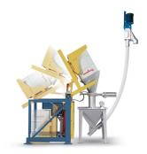
TIP-TITE® Drum/Box Dumpers seal, tip and mate a discharge cone to a gasketed hopper lid, open a slide gate and feed downstream processes automatically and dust-free.
