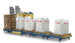
Flexicon Bulk Bag Filling Lines automatically dispense pallets, fill bulk bags, and disconnect/accumulate filled bags, minimizing operator involvement.
