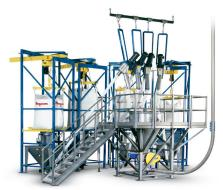
Enclosed Bulk Bag Weigh Batch Systems feed a central weigh hopper mechanically, and remove weighed batches pneumatically, requiring labor only to attach/detach bulk bags.
