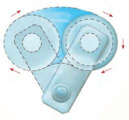
as the valve cycles, thereby shearing and wiping away any process material that may accumulate. No other valve is similar.
