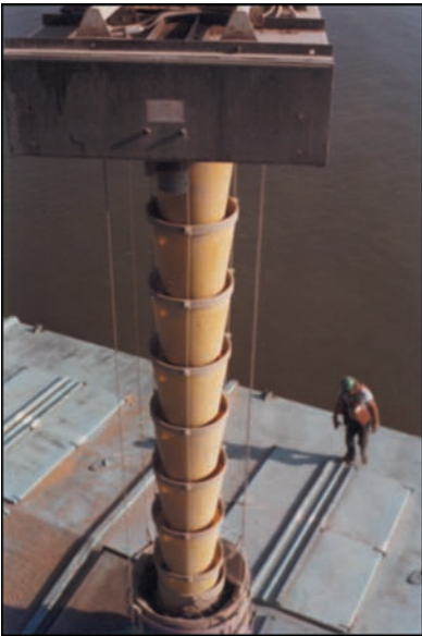
Heavy duty flex style spouts use inner cones to contain product flow enclosed by an outer sleeve for dust withdrawal. Inner cones are available in durable, lightweight urethane, 500 BHN carbon steel, or in stainless steel.
