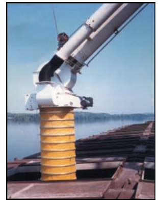
Pivoting gimbal allows different loading angles.
