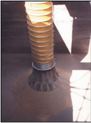
Dust free grain loading into barges.
