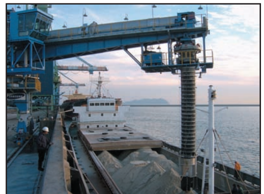
Model OV44 loading spout with model CFM470 loading kaolin clay.
