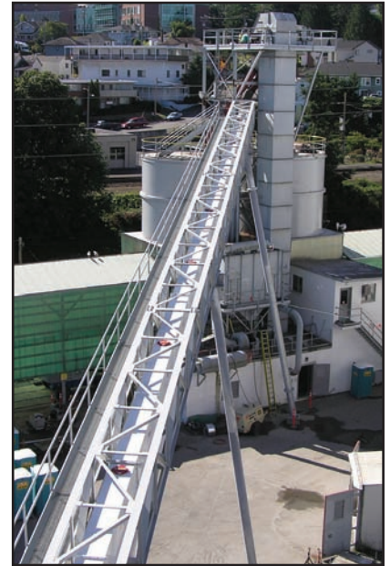
Aeration conveyor being fed by bucket elevator.
