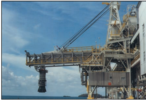
Model OV58 with combination boom and telescopic airslide for alumina loading.
