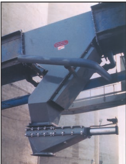
Aerated lump trap with slide gate valve.
