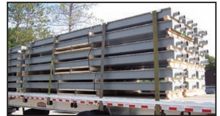
Aerated troughs for dome floor installation.
