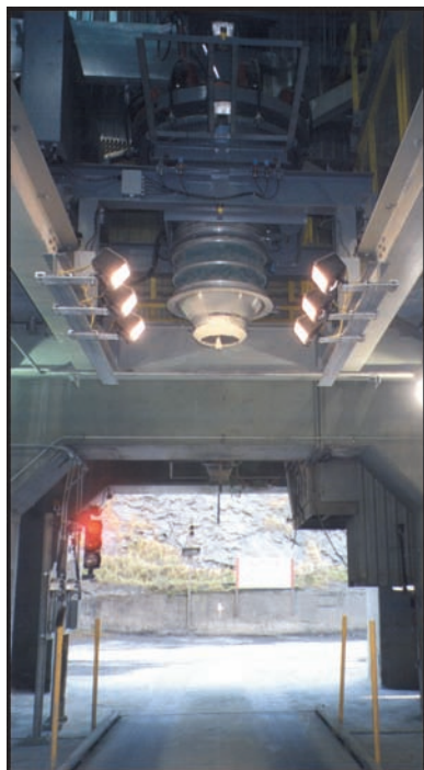
Typical equipment arrangement for fully automatic loading.
