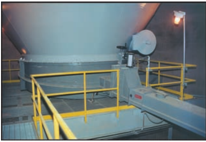
Aerated bin bottom discharging into a conveyor with slide gate valves.
