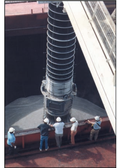
Dust free dry phosphate loading into ships.
