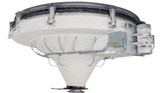
Prepared cake mix products are stored in activated surge hopper prior to packaging. Full diameter Bin Discharger creates uniform flow throughout the bin, remixing stored materials as it discharges. 304 stainless steel construction, white EPDM flexible connectors and white epoxy paint system meet FDA standards for bakery operations.
