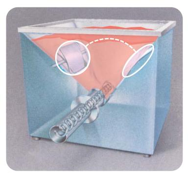
Diagram shows how continuous motion of the paddles on both sides of the hopper allows the agitation system to eliminate product degradation, rat-holing, bridging and compacting while handling the most difficult materials.
