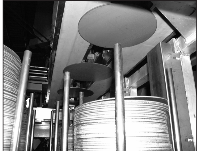
(A) Magnetic Transport Conveyor (B) Permanent Sheet Fanner (C) Bottom of hot water tanks
