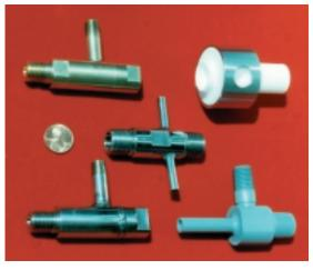
suctin ports, one with a special discharge connection, and a TFE unit armored with a protective ss sleeve.
